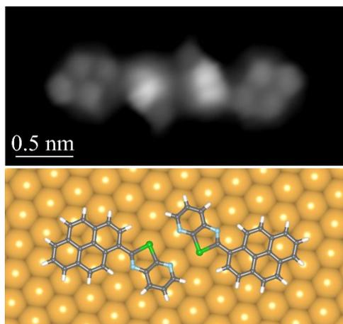
Fig. 1. BRSTM image of a dimer with double Se—N coordination (upper panel) and its geometrical model on an Au(111) substrate as optimized by DFT calculations (lower panel). Green balls represent Se atoms; cyan balls N atoms; grey and white balls C and H atoms respectively.
