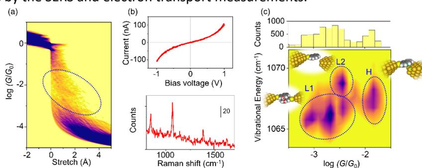
Fig.1. (a) 2D conductance stretch (b) typical  $I$ - $V$  curve (top) and SERS spectrum (bottom) for 2-NT SMJs obtained at  $10^{-3} G_0$ . (c) 2D histogram regarding vibrational energy of the ring breathing mode and conductance ( $G$ ).
